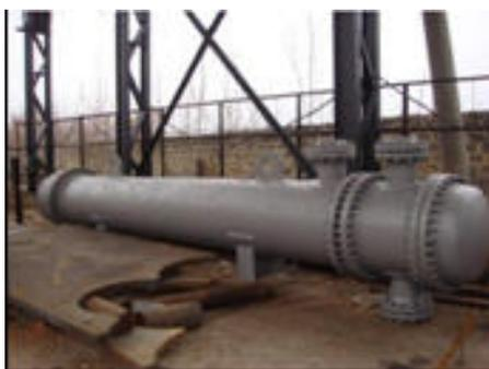
Titanium shell and tube heat exchanger
